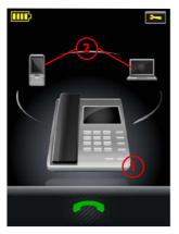
Current target phone: this large icon indicates the phone to which you will open a connection if you tap the headset multifunction button or touch the green handset icon at the bottom of the screen.
